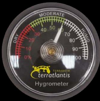
Hygrometer for precise monitoring of the humidity.
